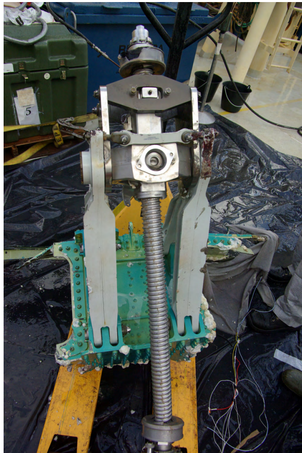
Trimmable horizontal stabiliser screwjack after being raised on board
