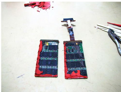
CVR memory boards after cleaning
