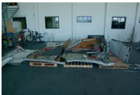
Floor of the LDMCR: with bottom-upwards deformation
