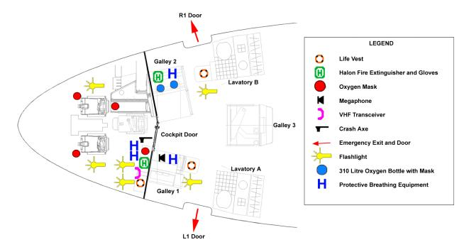
Figure 17: Emergency equipment location – cockpit and forward cabin
