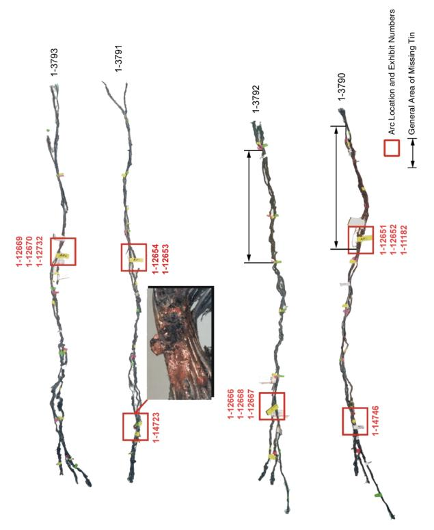
Figure 22: IFEN PSU cable segments
