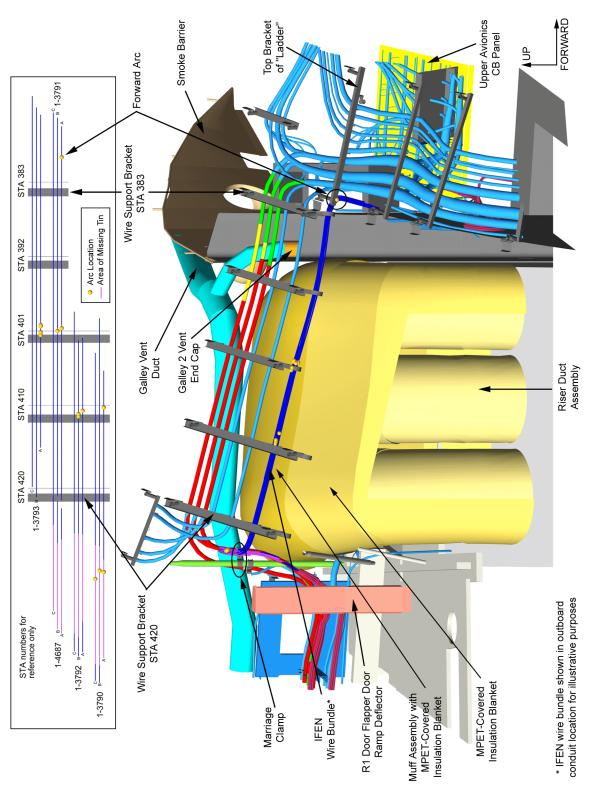
Figure 30: Position of recovered IFEN wires – outboard conduit
