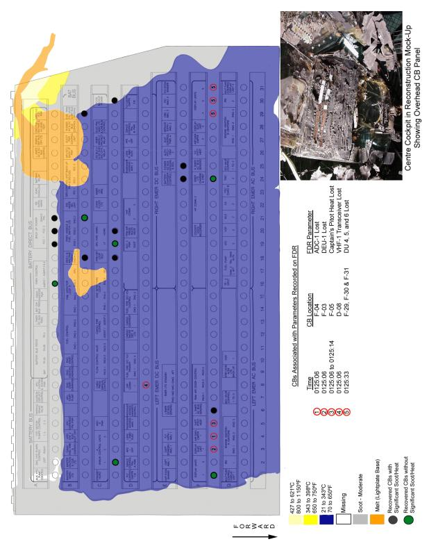
Figure 29: Heat damage – overhead CB panel
