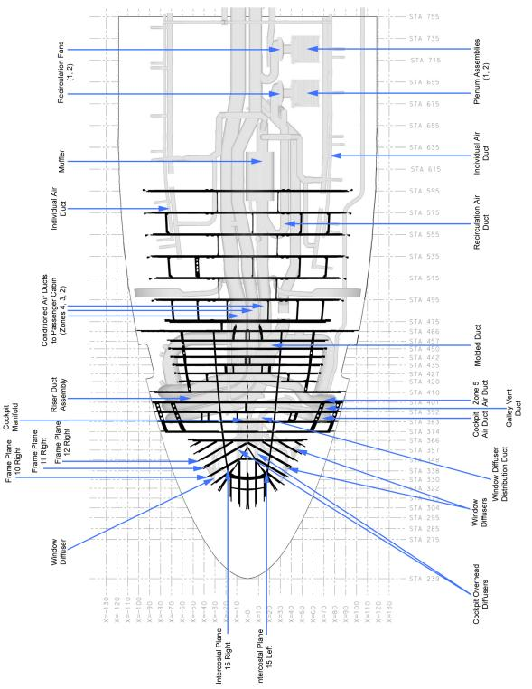
Figure 24: Airframe structure and air distribution system
