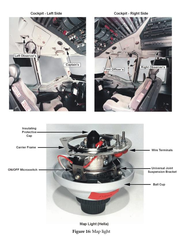
The Swissair MD-11 flight crew bunk module lights, PN 2LA 005 916-00 SWRA, were also manufactured by Hella. This bunk light was a map light that had been modified by removing the functionality of the ON/OFF switch to meet an FAA certification requirement. Although the bunk light used a different outer housing than the map light, the internal components were identical.
