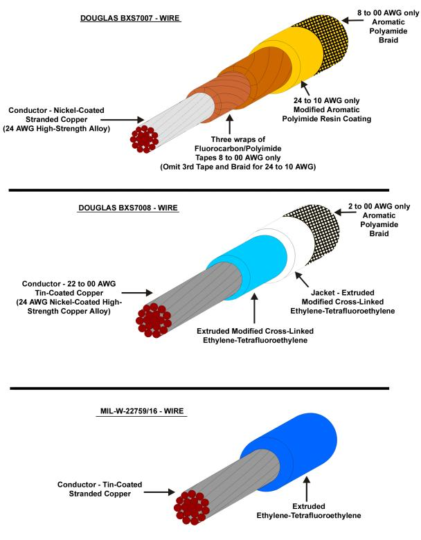
Figure 13: Wire construction
