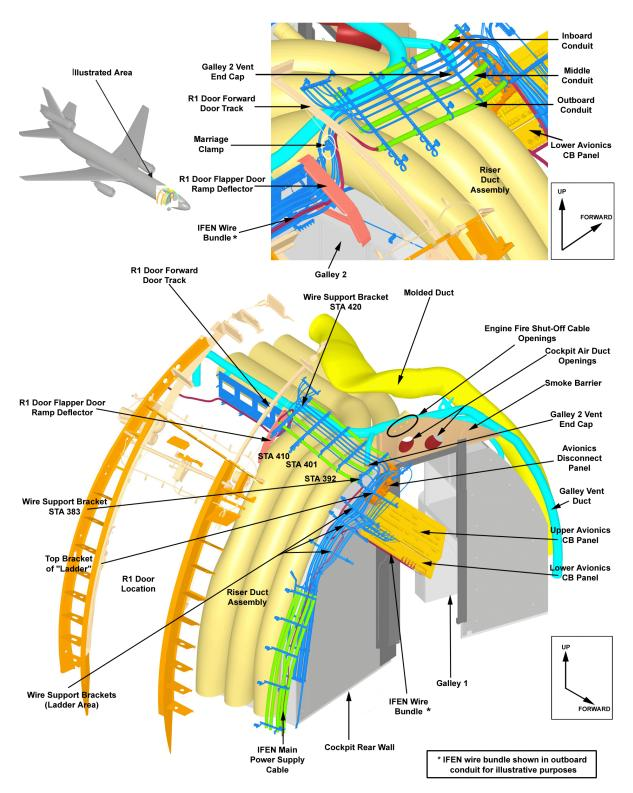
Figure 3: Cockpit attic and forward cabin drop-ceiling areas
