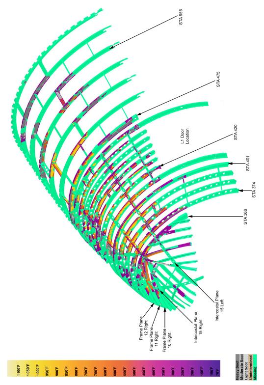
Figure 25: Heat damage – airframe structure
