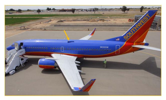
Figure 1. Photograph of N632SW with the hole in upper left fuselage.
