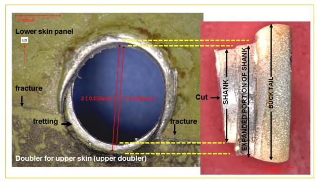
**Figure 6.** Rivet hole 85L when viewed from inner face of the skin panel (left side) and side view of corresponding rivet that was removed from the rivet hole (right side).
