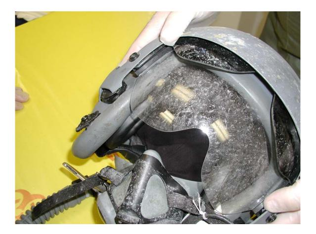
Photo 2 MDC Blast Damage
