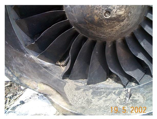
Photo 1 First Stage Compressor Damage
