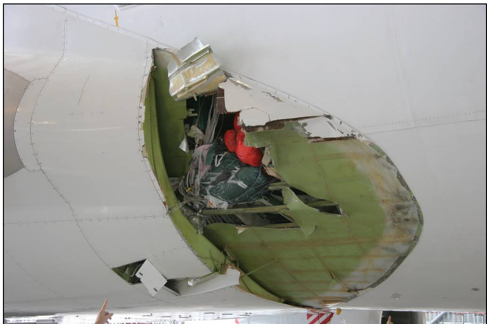
Figure 2: Fuselage rupture with protruding cargo
