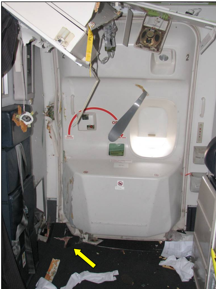
Figure 10: Interior of R2 door and cabin – location of floor hole arrowed
