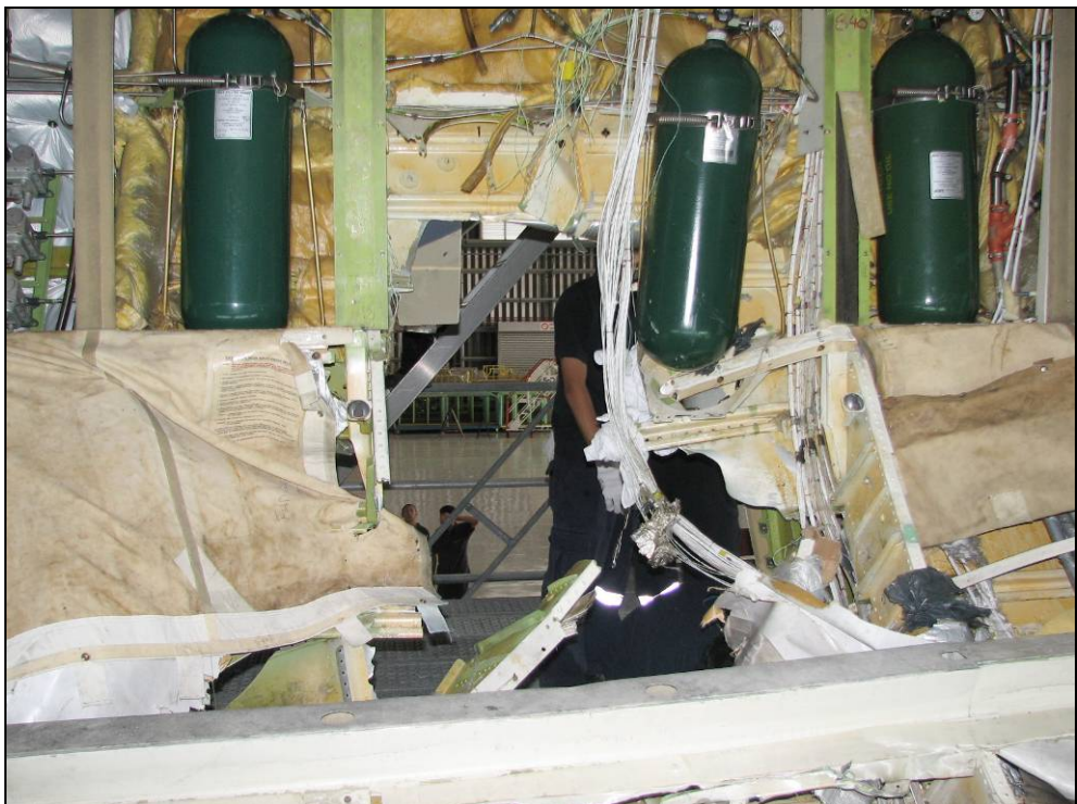
Figure 7: Fuselage rupture coincident with mounting position of the number-4 oxygen cylinder
