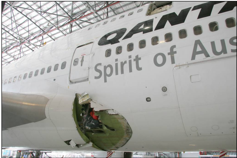
Figure 2: Fuselage rupture with protruding cargo
