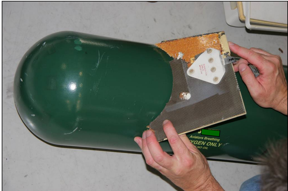
Figure 17: Semi-circular damage in partition of compartment above R2 door
