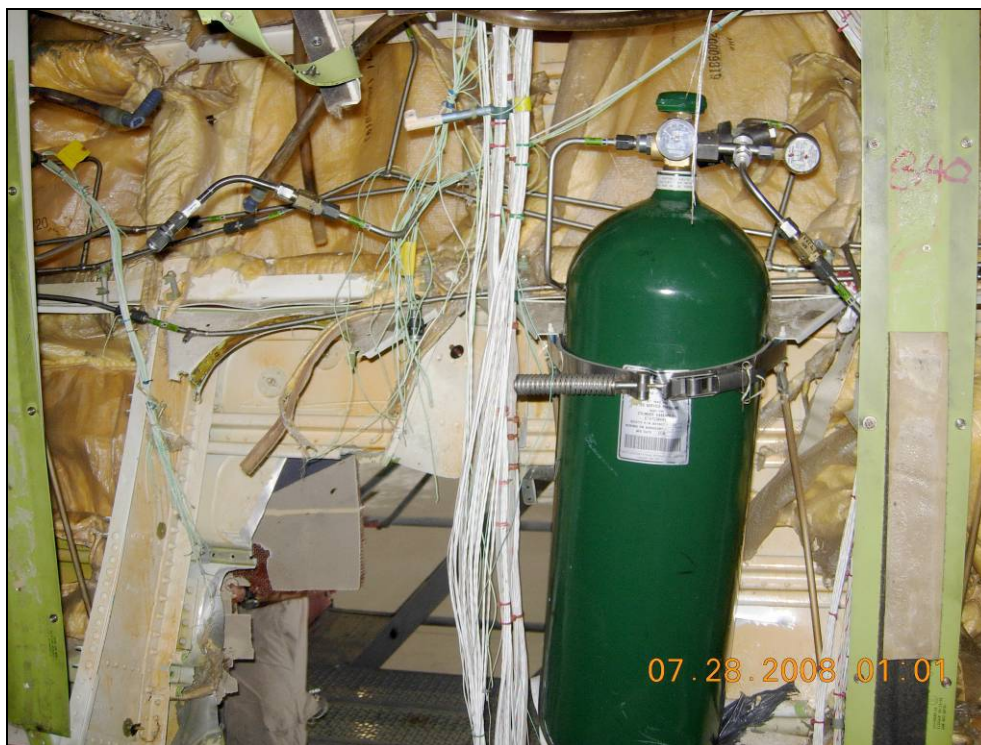
Figure 8: Number-5 oxygen cylinder adjacent to fractured fittings and lines from the number-4 cylinder
