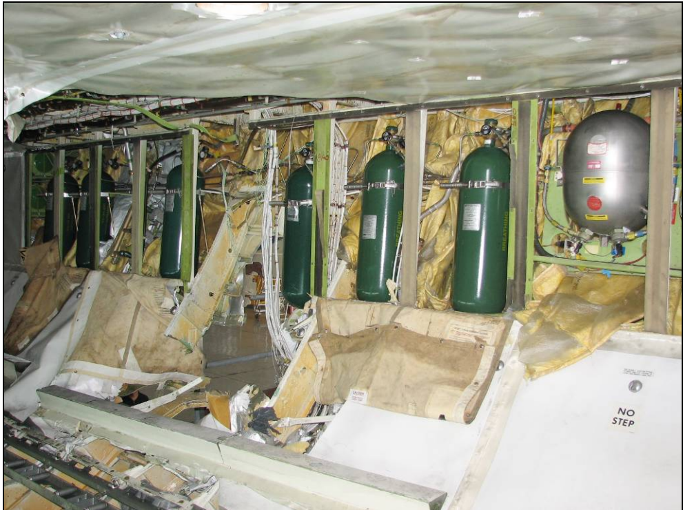
Figure 7: Fuselage rupture coincident with mounting position of the number-4 oxygen cylinder
