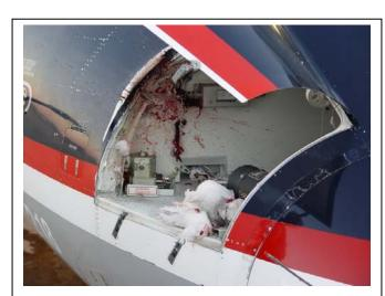
A CRJ 200 descending into a southern USA airport hit a flock of snow geese, 27 November 2007. Aircraft landed safely, but inspection revealed major damage to multiple components including 1 engine, nose, wing root and horizontal stabilizer.
