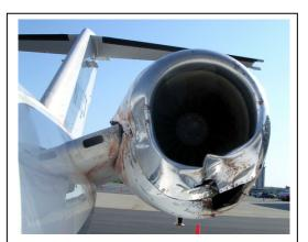
A Cessna 525 en-route at 5,000 feet AGL hit a flock of white-winged scoters, 21 May 2007. An emergency landing was made at a northeastern USA airport. Both engines, the windshield and fuselage were damaged.
