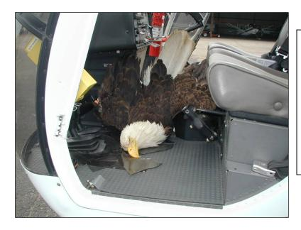
A bald eagle shattered the windshield of a Schweizer 300 helicopter at 2,000 feet AGL in Minnesota, 3 June 2007. The passenger was knocked unconscious and suffered cuts and bruises. Pilot landed the aircraft safely with the dead eagle at his feet. Photo, Chris Cooper, Hummingbird Helicopters.
