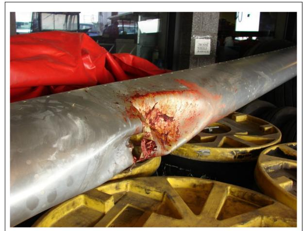
The leading edge of left wing of a B-737 hit a great blue heron on approach to an east coast USA airport, 7 November 2007. The pilot landed the aircraft uneventfully where it was taken out of service for repairs.
