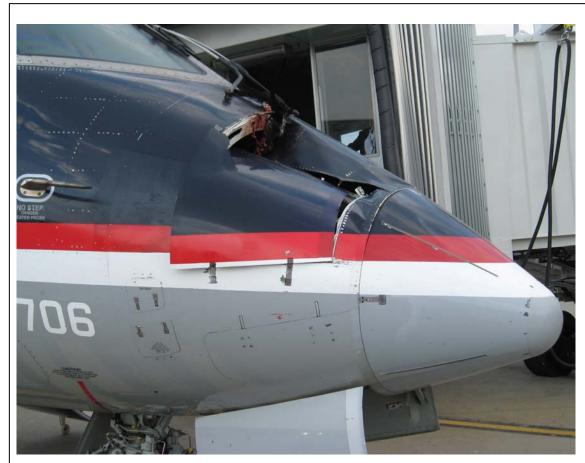
A CRJ-700 struck a black vulture on final approach to an airport in Kentucky on 28 August 2007. The strike caused substantial damage to nose cone. The black vulture population in USA increased at a mean annual rate of 2.6%, 1980-2006.
