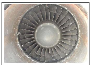
A Learjet 36 ingested a mallard into an engine during the takeoff run at a northern USA airport, 4 June 2007. Pilot aborted takeoff. Cost of repairs was >\$250,000.
